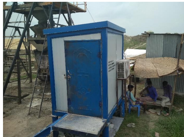
6. Batching plant's operator room with AC
