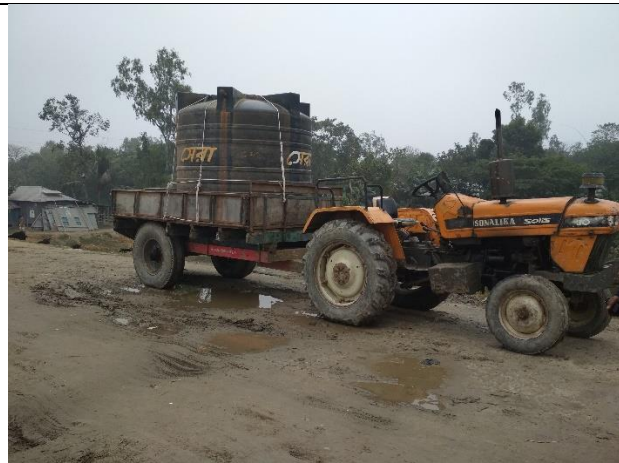
4. Water is being spraying through machine for dust suppression
