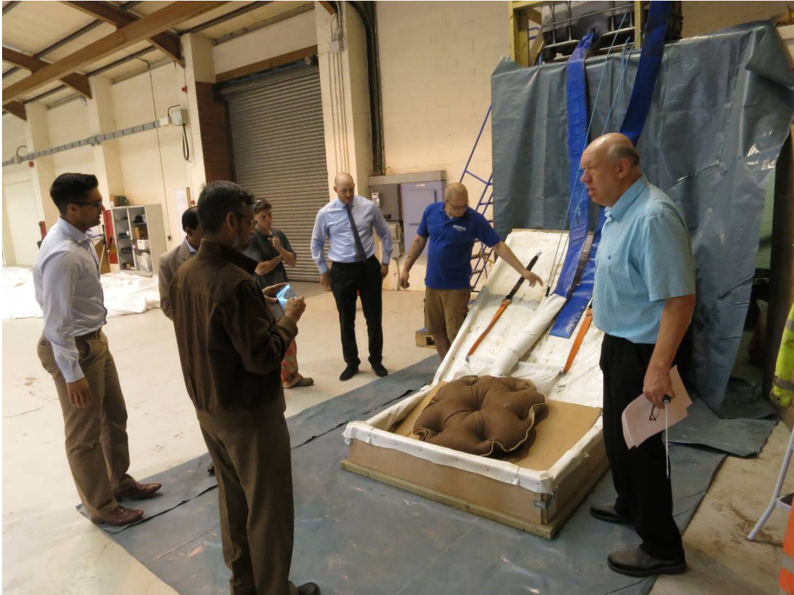
Figure 2. Demonstration of grout filled mattress section made of jute fibers
