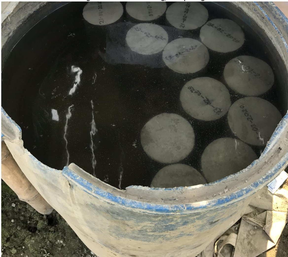
Figure L 15: Concrete cylinder curing for concrete cylinder compression test, W16 package
