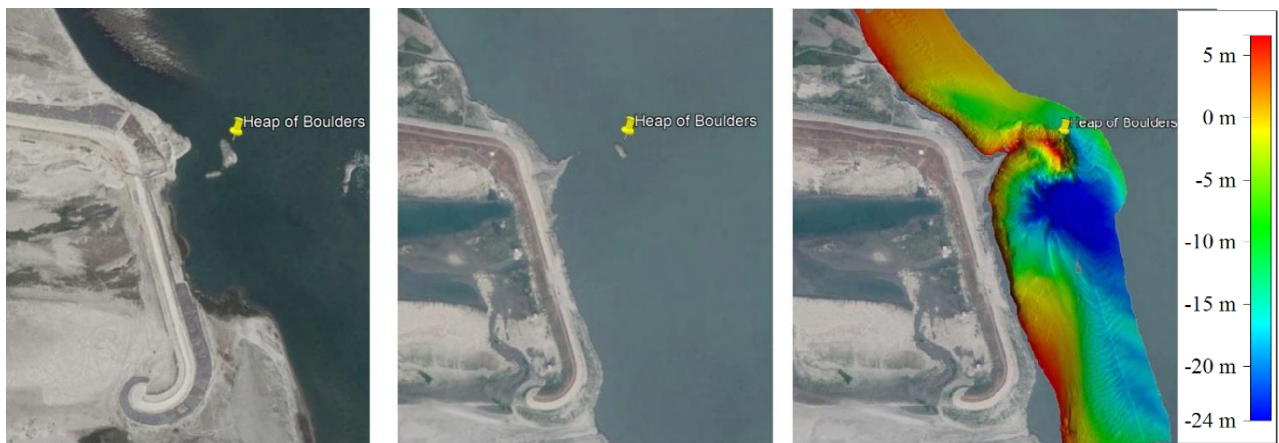
Figure 4-8 Bathymetry near Sirajganj cross bar
